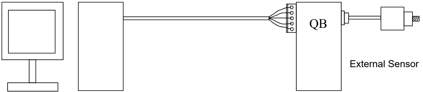
Figure 13: Terminal Block - Second Loop with Combined Data and Power Cables
