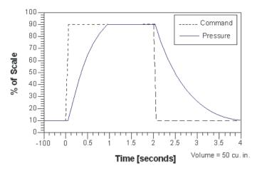
Times for QB3 to fill/exhaust a closed chamber. Time is determined by difference between command signal and pressure achieved.
