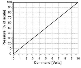
Linear characteristics for a QB3 when given a ramp signal from 0-10 volts. Characteristics would be similar for 4-20mA units.
